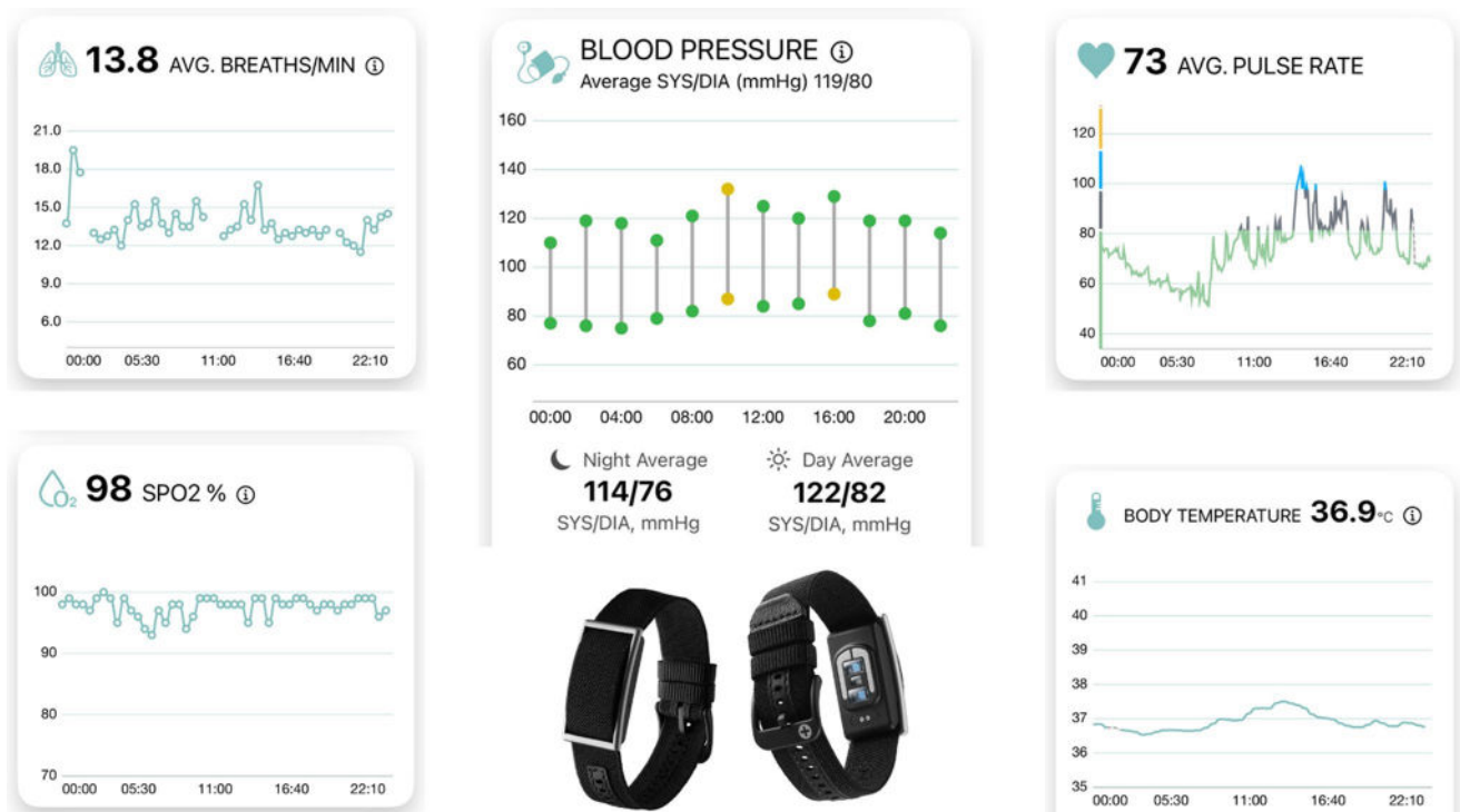
Fig. 2 Example of medical-grade photoplethysmographic wristband enabling the semi-continuous monitoring of 5 vital signs. Abbreviations: AVG., average; SYS, systolic pressure; DIA, diastolic pressure;
