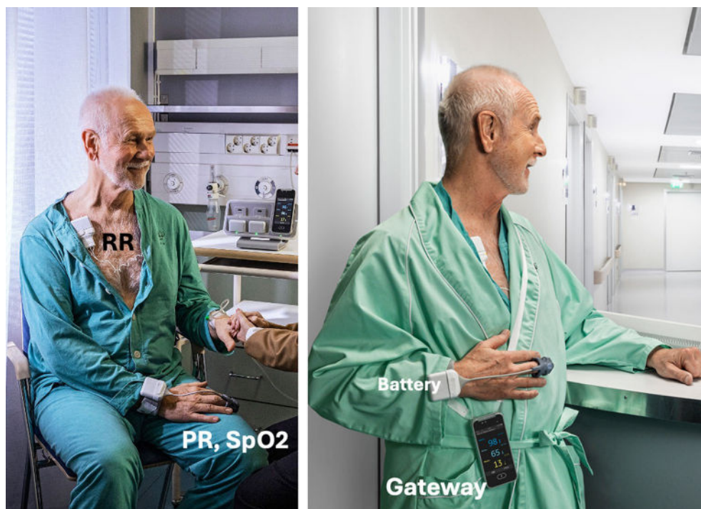
Fig. 1 Example of mobile monitoring system using chest and abdominal electrodes to compute respiratory rate (RR) from cyclic changes in thoracic impedance, and a finger photoplethysmographic sensor to monitor oxygen saturation (SpO 2 ) and pulse rate (PR). Continuous data transfer to the gateway (a smartphone-like device following the patient) is secured by a proprietary connectivity protocol. From GE Healthcare with permission
