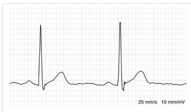
ECG signal after Pan-Tompkins QRS detection and filtering
