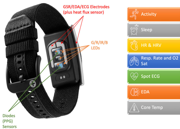
Fig. 1 The Corsano 287-2B. Sensors and metrics available from the medical-grade wearable used by students 21 .
