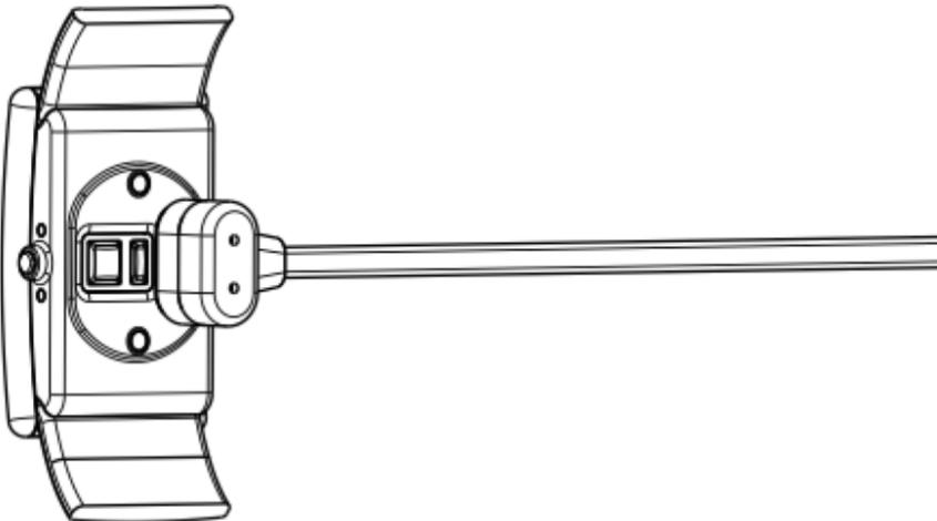
*Figure 7 – Charging view – charger attached*
