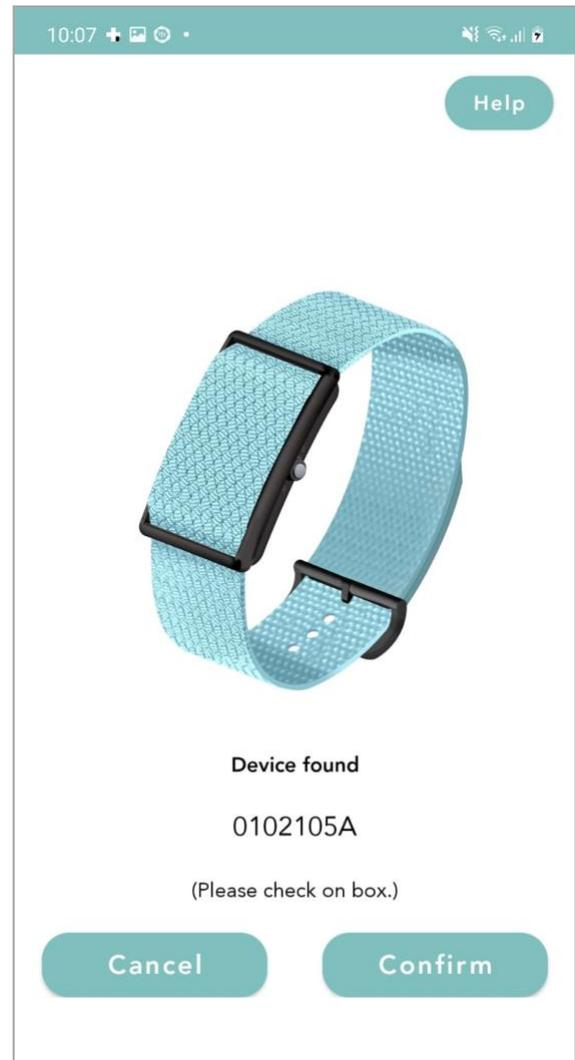
Once the device is found, confirm by pressing on the pusher. On successful pairing, the bracelet will light the orange LED up for 10 seconds and then turn it OFF.
